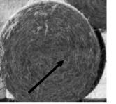
Round bales have to be measured on the face side. Measurements at the bearing surface lead to miss readings.
